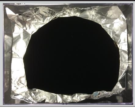
Developed by Surrey NanoSystems, Vantablack is a super-black coating that holds the world record as the darkest man-made material. Vantablack absorbs up to 99% of visible light. Composed of vertically aligned carbon nanotubes, Vantablack literally traps light which is continually deflected within the tubes until it becomes absorbed.
