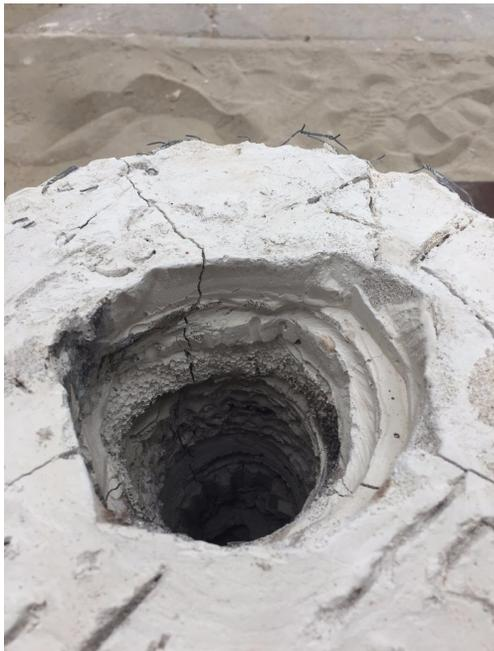
*Lost-wax mold after kiln burnout.*
