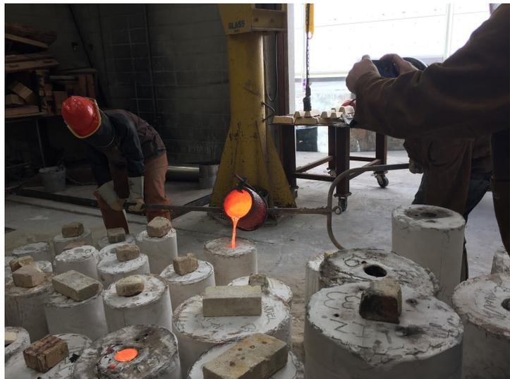
*Pouring molten metal into mold.*
