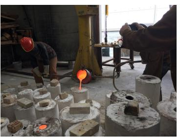
Pouring molten metal into mold.
